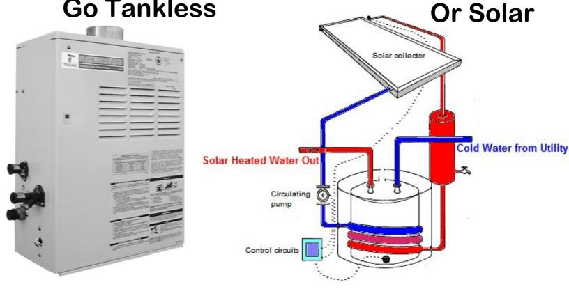
Tankless water heaters don't store hot water. They generate it on demand. "Solar" heats water using the sun, and is the most cost-effective method of heating water!
