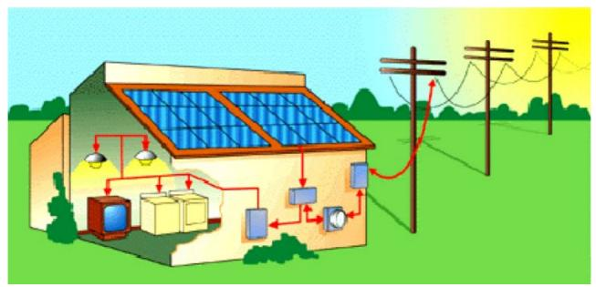
Power generated by the solar modules on the roof is converted to household electricity, slowing the meter.
